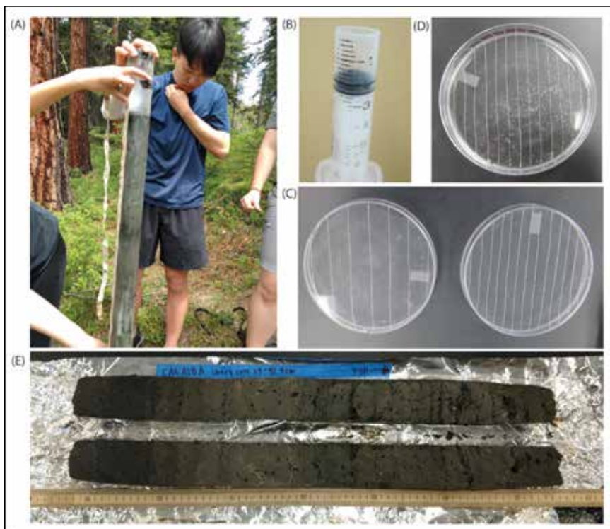
Figure 2.—Images showing (a) Lightning Lake LNL12B sediment core, (b) modified syringe used to sample sediment for MCA, (c) scored petri dishes used in MCA, (d) sediment residue in petri dish after processing and sieving, (e) Camp Lake CALA18A sediment core split longitudinally.
